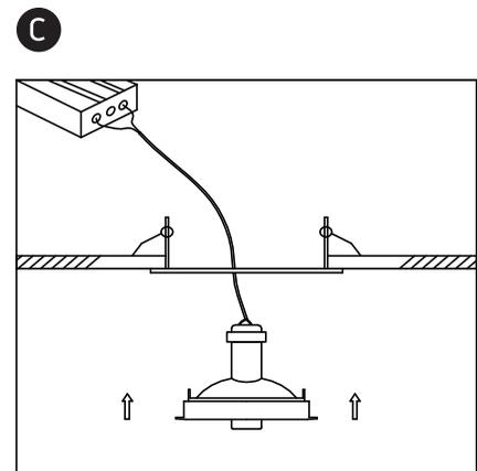
\*Insert the complete module into the base.
