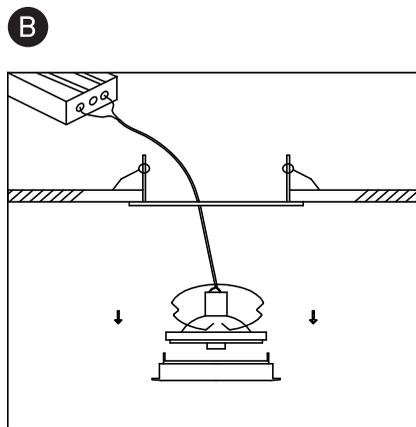
\*Insert the corresponding lamp into desired module.
