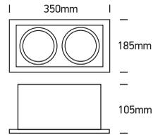
230V | COB LED | 2x30W | IP20 | Aluminium + metal
